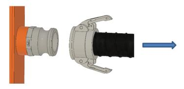
2. Unlock the pin and remove the suction cup
